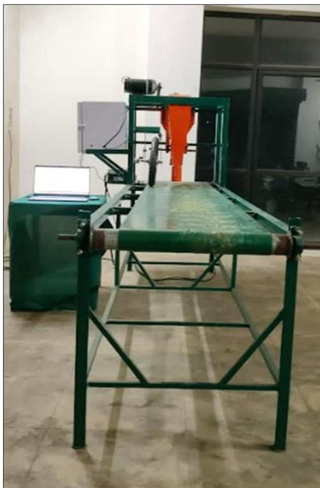
Fig 10: Developed laboratory set up for the sensor-based tractor drawn ginger planter
