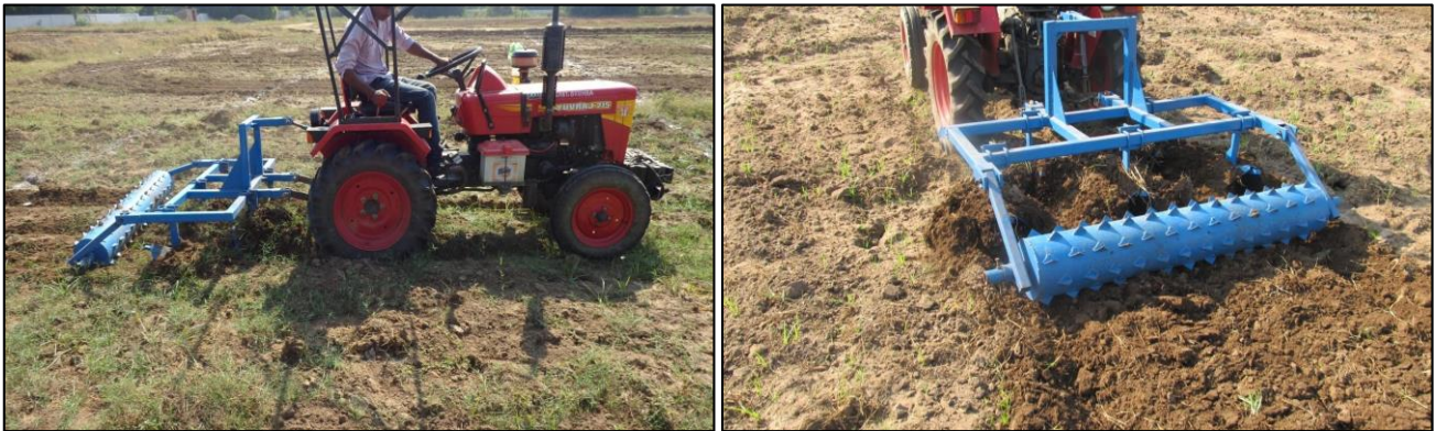
Plate 1: Multi purpose tillage implement with clod crusher during operation
