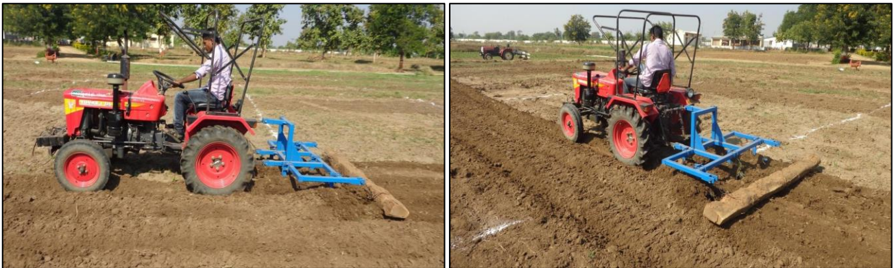
Plate 2: Multi purpose tillage implement with Planker during operation
