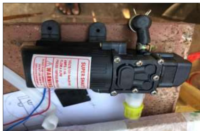
Fig 4: DC Motor pump
