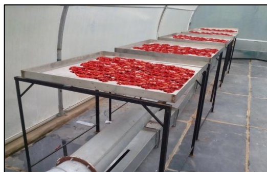
Fig 2: Drying of nutmeg mace in solar tunnel dryer with biomass backup
