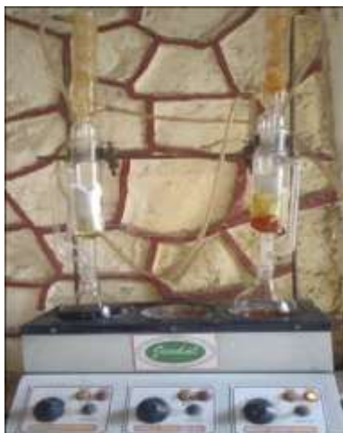
Fig 3: Photograph showing preparation of ethanolic extract of stem powder of Tinospora cordifolia and root powder of Glycyrrhiza glabra by Soxhlet apparatus
