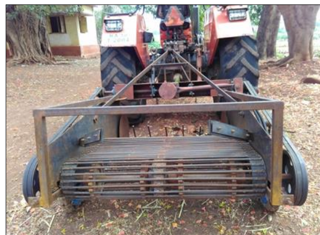
Fig 1: Developed tractor drawn ginger harvester-cum-elevator
