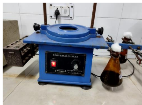
Fig 3: Electric shaker used to properly mix Butea monosperma leaf powder with methanol.
