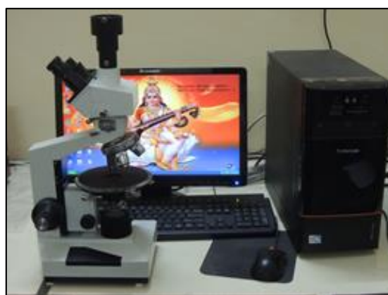
Fig 2(a): Optical Study Setup: Polarized Light Microscope (PM) coupled with digital Camera made by CENSICO (India).
