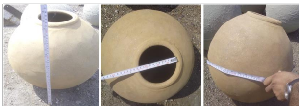
Fig 1: Dimensions of pots used in black salt manufacturing
