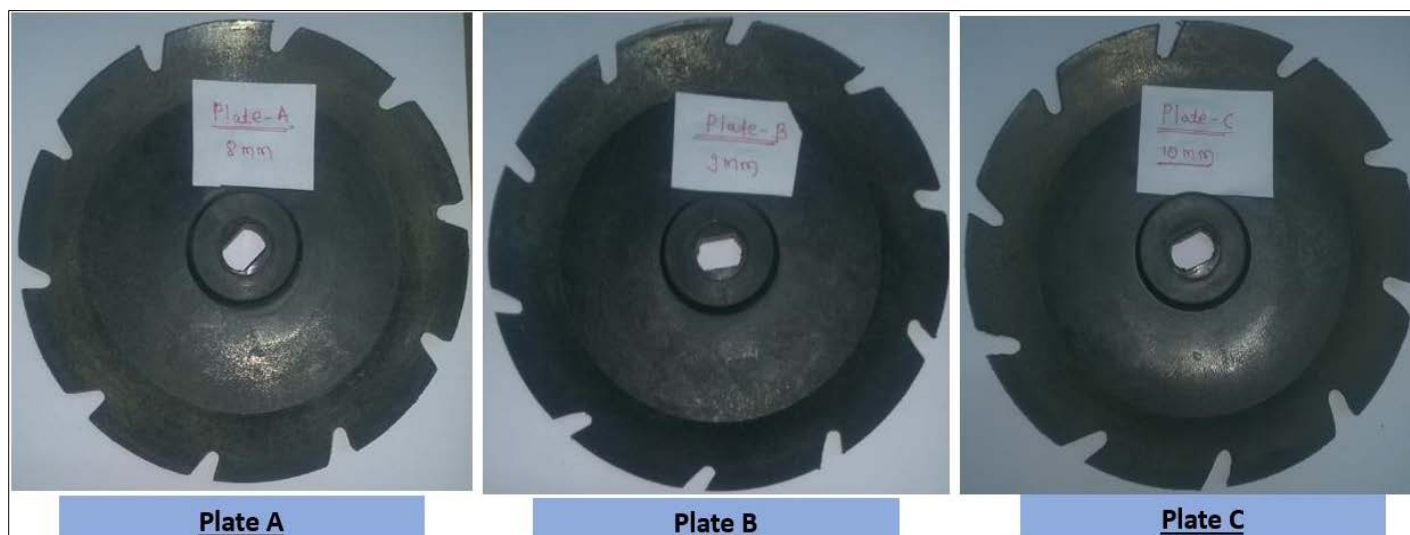
Fig 2: Metering plates used for metering of soaked okra seeds
