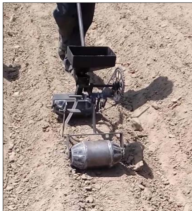
b) Working operation of ridge vegetable planter
