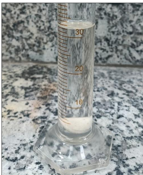
Fig 4: Hexane displacement method for calculation of true density
