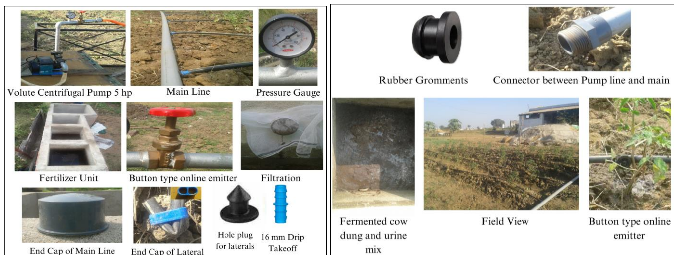
Fig 1: Components of organic drip fertigation unit
