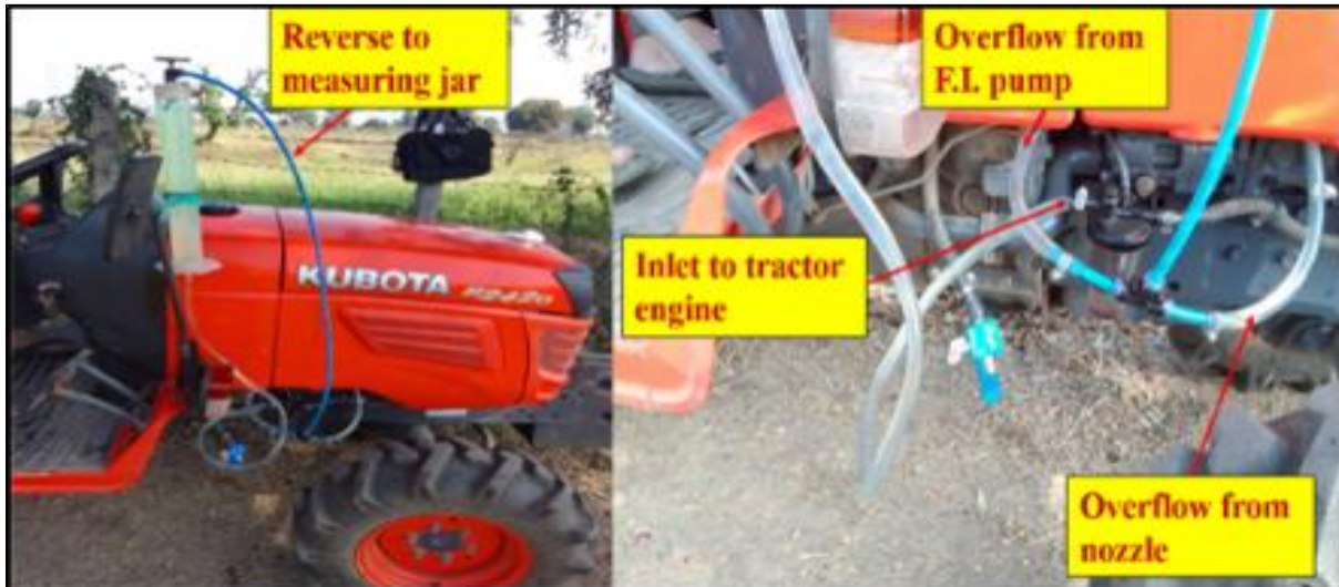
Fig 1: Setup of Fuel Consumption Measurement
