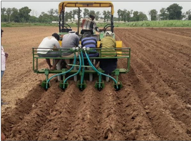
Fig. 3: Sowing operation of turmeric with 4- row seed drill (ridge and furrow method)
