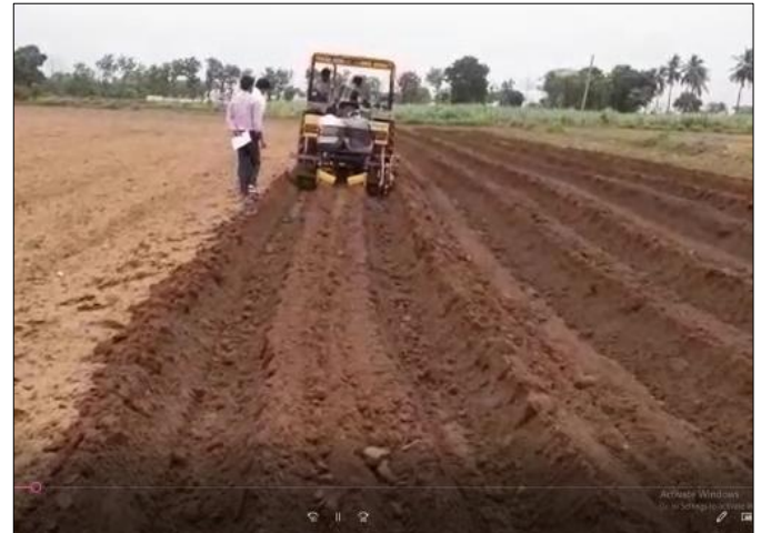
Fig 4: Sowing operation of 2- row raised bed turmeric semi-automatic planter
